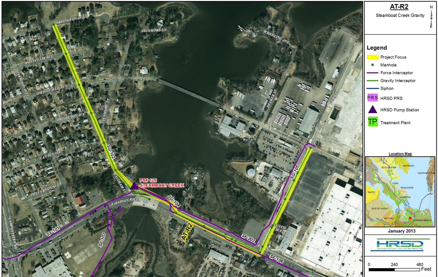
Figure 4-6. Project AT-R2. Steamboat Creek. Sheet 4 of 4.
